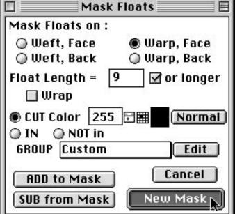
Each warp-face floater shows up as a vertical column of 9 (or more) black pixels. Each floater can be fixed by changing one those black pixels to a non-black color - which will break it into 2 shorter warp-face floats by forcing the warp the leave the front to cross under a weft.
